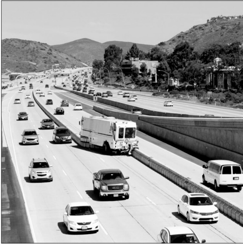
Road Zipper by Lindsay Corp. of Omaha is a way to lift barriers that can more easily reconfigure travel lanes. The zipper was a contestant in the 2022 Coolest Thing contest. (Courtesy of Nebraska Chamber and Nebraska Manufacturing Alliance)
